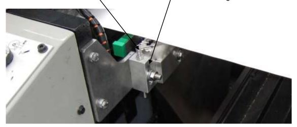
c. The manifolds have to be adjusted to the web that the ends of the brushes touch the web.
