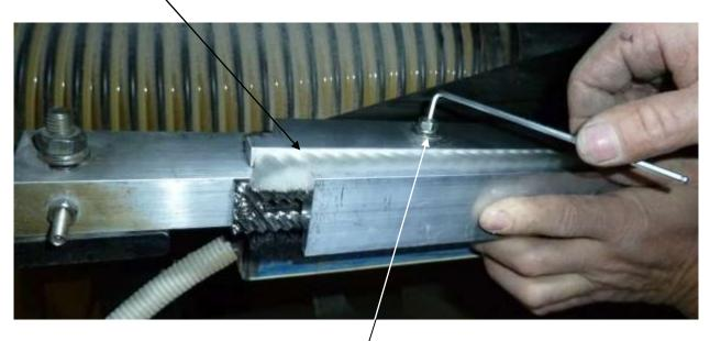
Push the inaccesible brushes against the template through the movement of the eccenter screw with the socket wrench.
