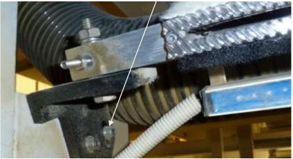
b. The manifold hast o be parallel to the web. If this is not the case, the brushes are wearing off differently from side A to side B and it is not guaranteed the brushes fulfill their tightening function (vacuum).
